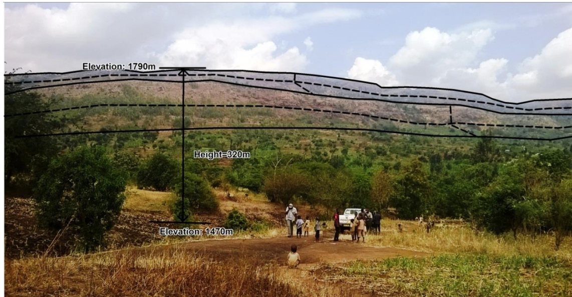
Figure 9: Photo showing how the height of the Nasho quartzite was measured.
